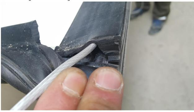
4) After heating cable removal, insert new cable. Connect it to the box. Glue cut parts of gasket.
