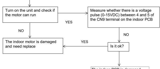
The indoor PCB is damaged and need replace
