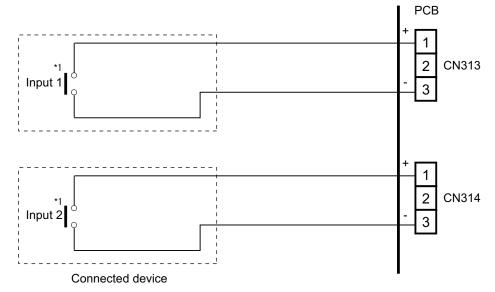
\*1: The switches can be used on the following condition: DC 12 V to 24 V, 1 mA to 15 mA.
