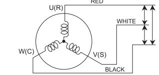
$\rightarrow$  If the resistance value is 0  $\Omega$  or infinite, replace compressor.
