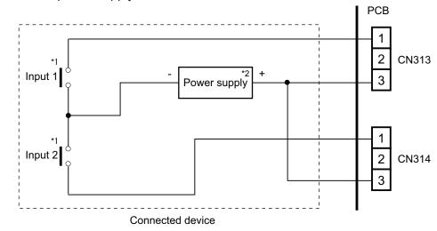
\*1: The switches can be used on the following condition: DC 12 V to 24 V, 1 mA to 15 mA. \*2: Make the power supply DC 12 V to 24 V, 10 mA or more.
