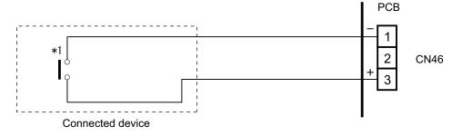
\*1: The switch can be used on the following condition: DC 12 V to 24 V, 1 mA to 15 mA.
