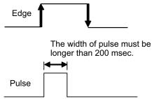
**NOTE:** The input signal supports the following switch type:
