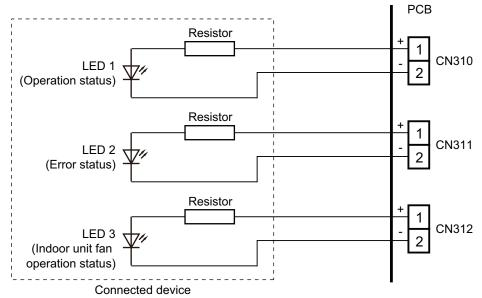
When connecting with a device equipped with a power supply: Example: Rotary SW on External Input and Output PCB is set to "1".
