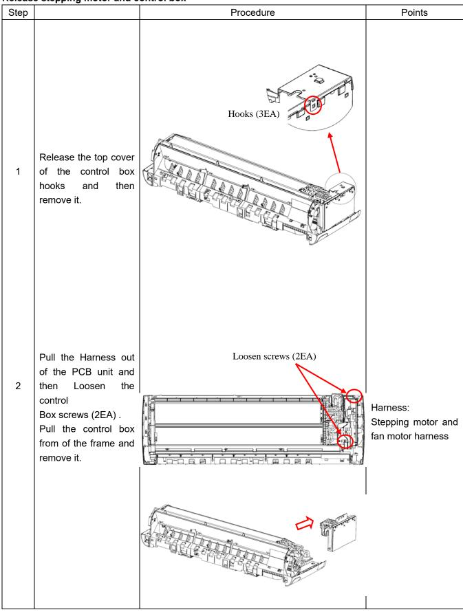
Release stepping motor and control box
