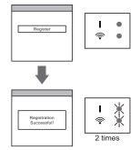
Both of the LED 1 and 2 flash 2 times and a message appear when the setup is completed.
