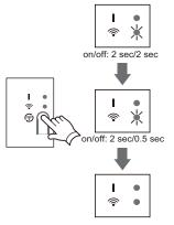
The light pattern of the LED 2 changes. (On/off: 2 sec./2 sec.  $\rightarrow$  2 sec./0.5 sec.) Confirm both of the LED 1 and 2 are on to proceed.
