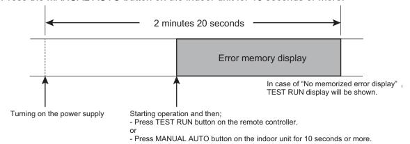
\*: The "3 minutes ST" period lasts 2 minutes and 20 seconds after turning on the power supply.
