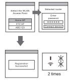
When setup is completed, both of the LED 1 and 2 flash 2 times and a message appear.
