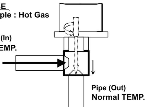
If it is open, it has no temp. difference between inlet and outlet
