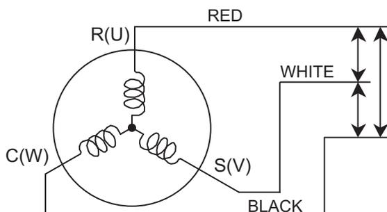
→ If the resistance value is 0  $\Omega$  or infinite, replace the compressor.
