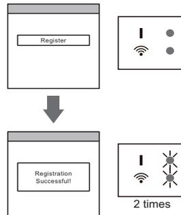
Both of the LED 1 and 2 flash 2 times and a message appear when the setup is completed.
