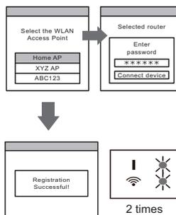
When setup is completed, both of the LED 1 and 2 flash 2 times and a message appear.
