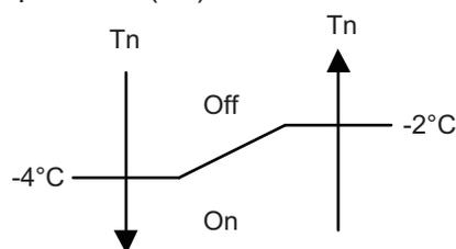
When the jumper wire (JM2) is disconnected:
